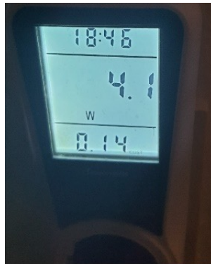
Figure 2: Display of watt meter showing current Wattage in the center of the display
